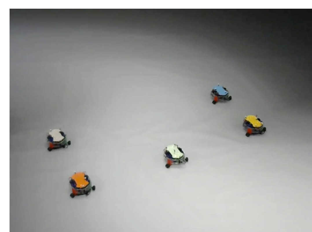
Five mini-robots navigating down a ridge in a laboratory testbed.
