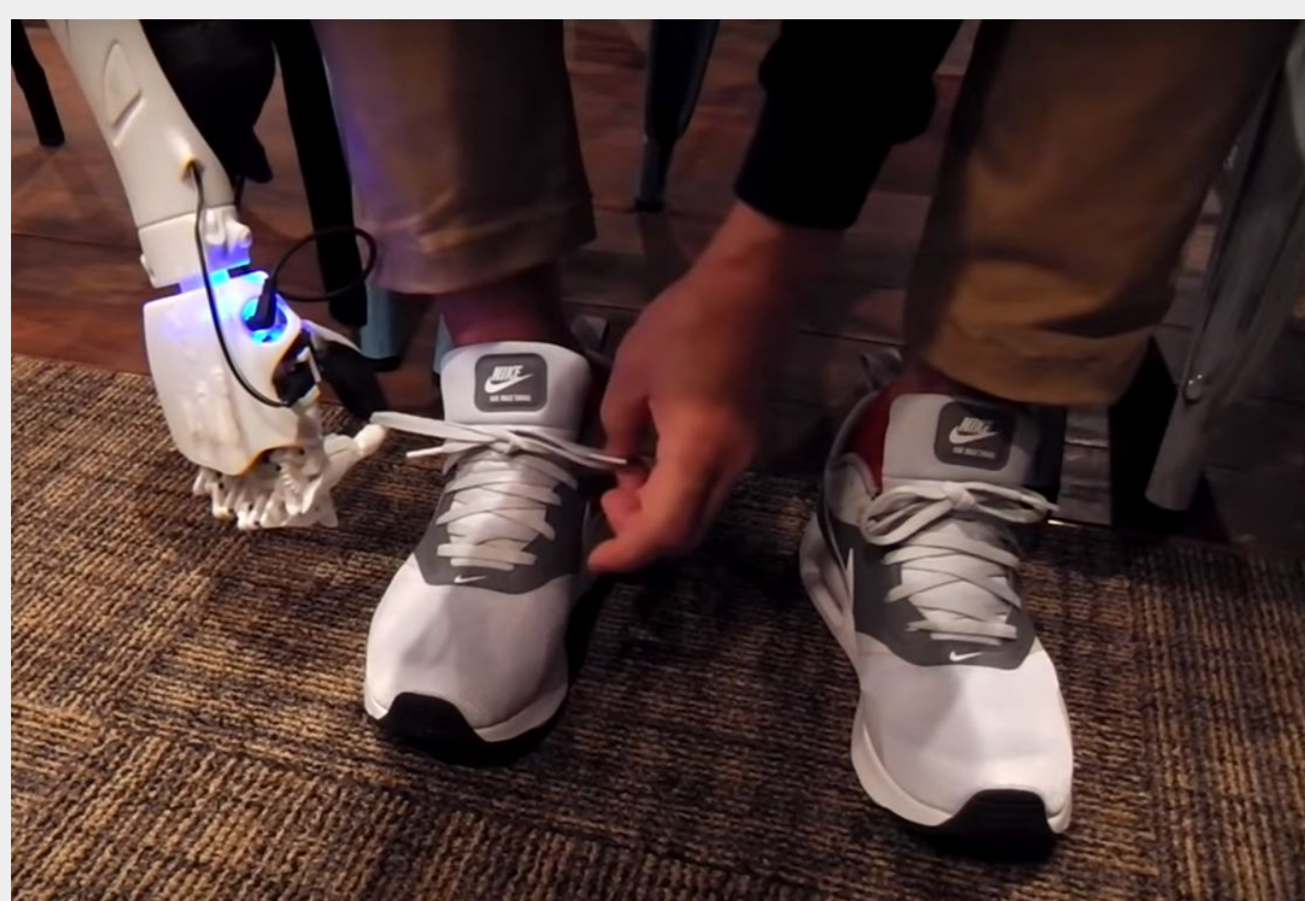
Image 1: A prosthetic arm, the HACKberry, allows a man to tie his shoes [2].
