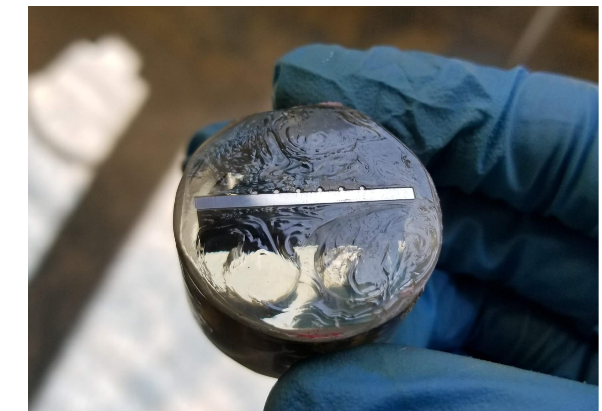
Figure 9 Wire bonded sample after the first alumina polishing steps
