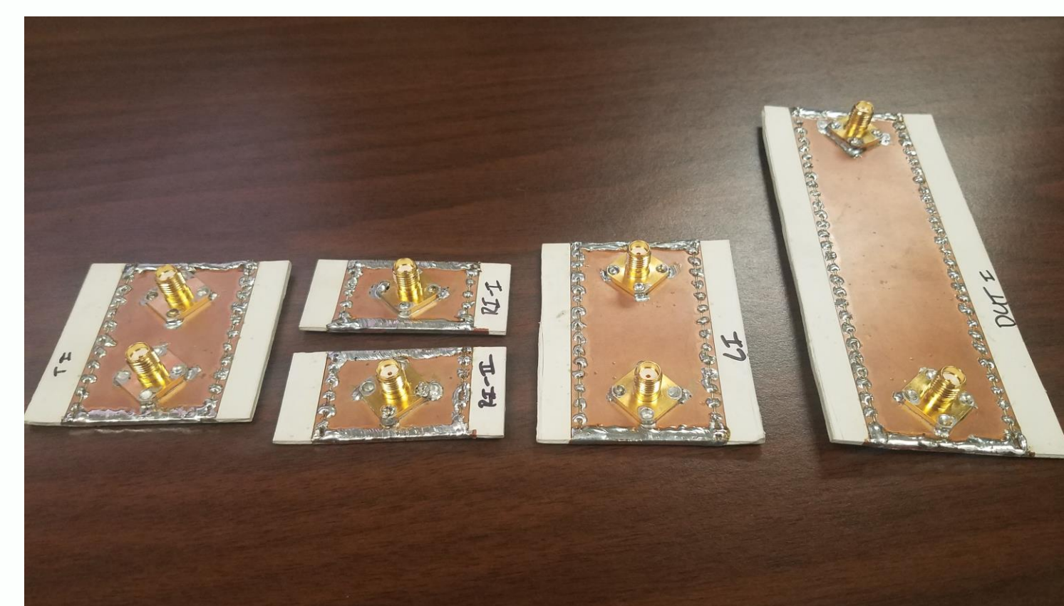
Figure 5: From left to right: TRL calibration standards (through, reflect, line) and example device
