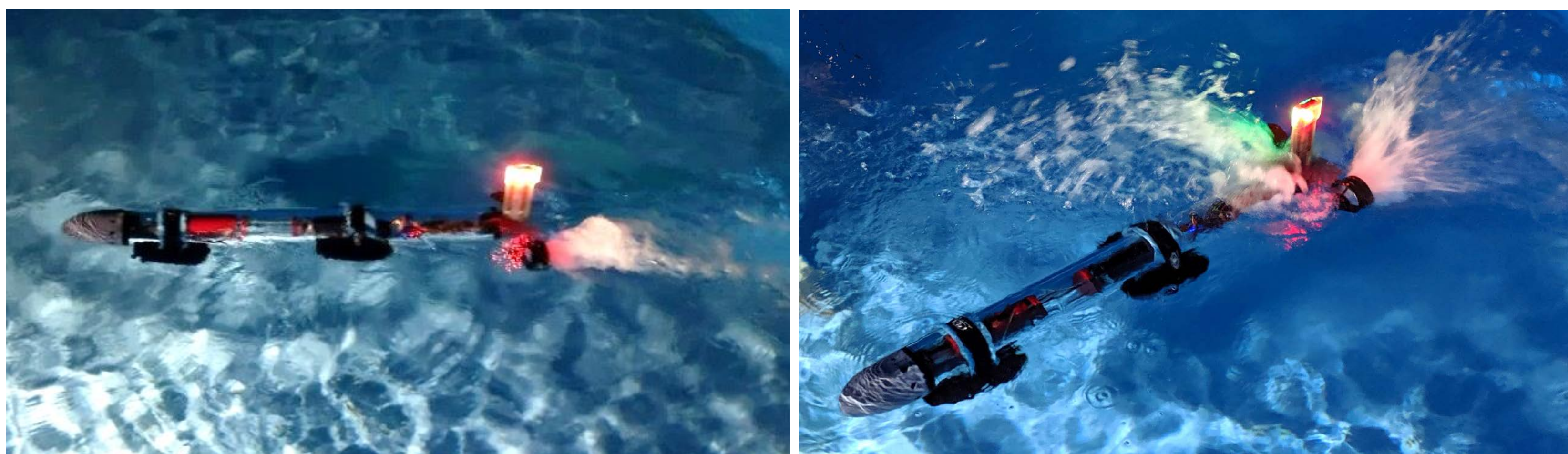
In-water actuator tests: transit (left), starboard turn (right)
