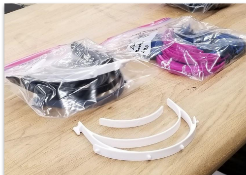
Mass produced 3D printed parts for face shields for medical personnel
