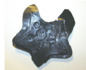
FLASHING & SINK MARKS
