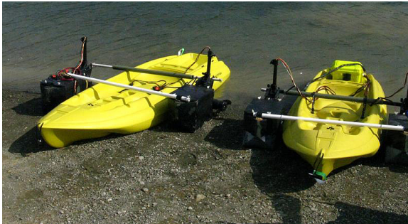
FIGURE 6. Autonomous surface vehicles with propulsion systems and custom sensor and communication suites.
