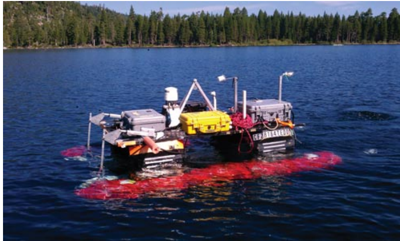
Figure 1. The Santa Clara University SWATH boat operating automatically during a bathymetric mission in Lake Tahoe, CA.
